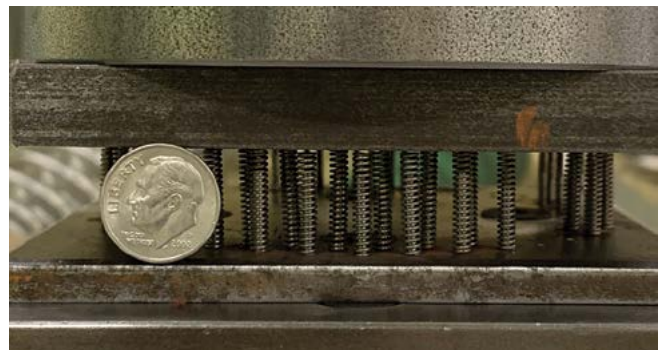
Figure 2 - Test fixture capable of cycling 70 springs simultaneously.
