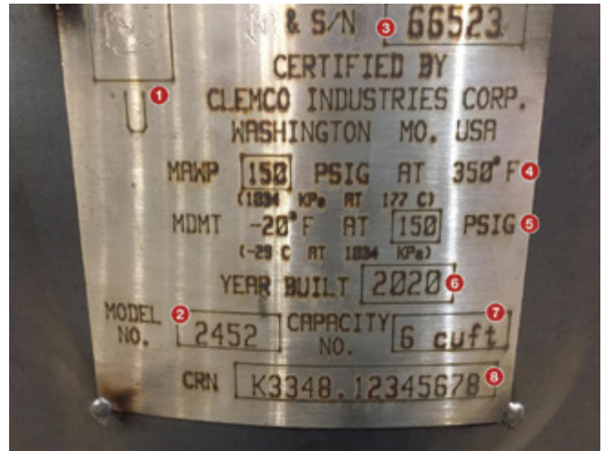
Every Clemco pot has a U or UM stamped on its compliance plate, which certifies that it has met ASME design, construction, and inspection requirements
