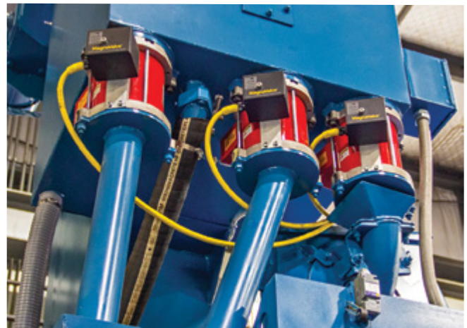
The 500-24 MagnaValve and FC-24 Controller regulate the flow of steel shot in the 72T Shot Peening Table
