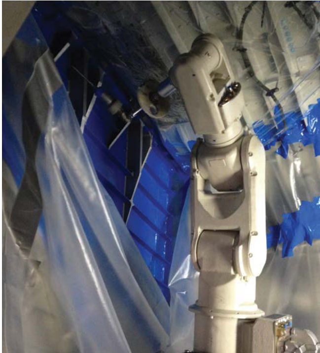
Figure 2: Robotic peening of critical geometry
