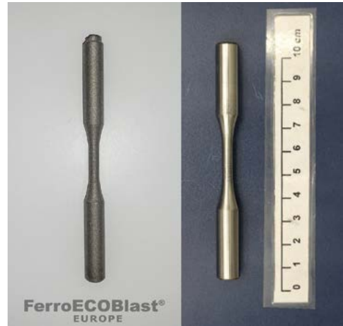
Figure 1: Test subject – 3D printed test piece Left: Raw, untreated part • Right: Ground, before shot peening
