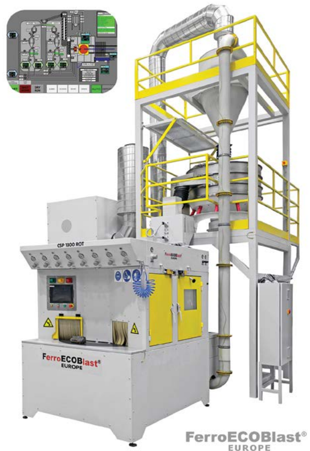
Figure 8: One of FerroECOBlast's many automatic shot peening machines
