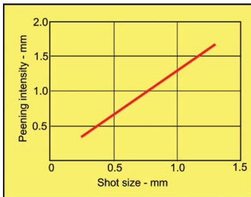
Fig.4. Peening intensity versus shot size.
