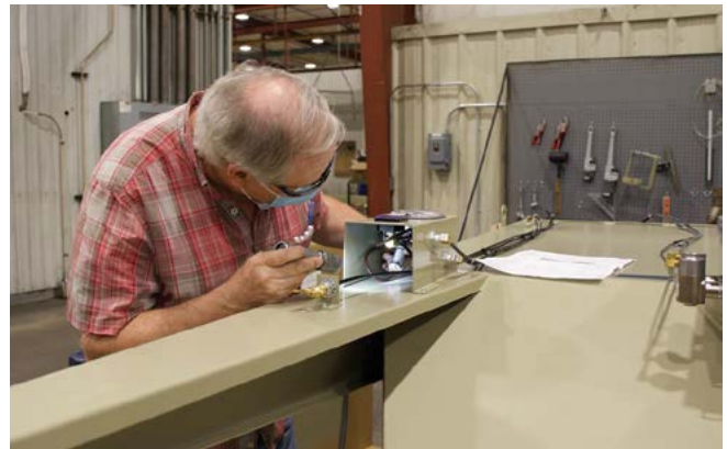
Rick examines an RPH-2 Dust Collector's magnehelic gauge for air leaks and proper connections as part of the Factory Acceptance Program's 62-point inspection checklist.
