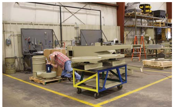
Rick checks that the dust-collector motor is rotating correctly and that the motor-housing welds are secure.
