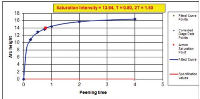
Fig.9. Peening intensity calculation using a three-parameter equation.
