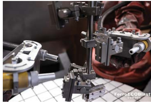
Universal Almen strip holder for intensity check during Factory Acceptance Testing of the ARSP 1000 ECO DUAL machine
