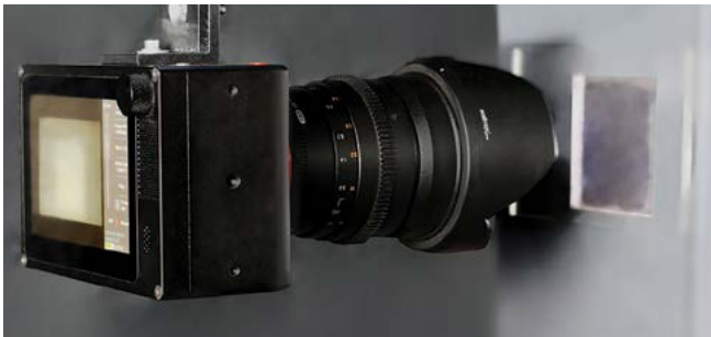
High-speed camera installed on a peening machine window
