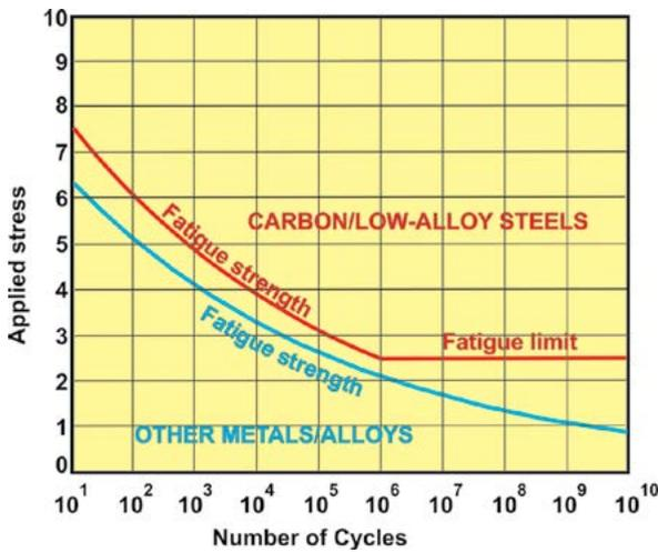
Fig.3. Two shapes of fatigue curves.
