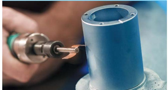
*Rotary flap peening is ideal for peening small areas on new or repaired parts. The process can be done in the field, eliminating the time-consuming and expensive disassembly and transportation of components.*
