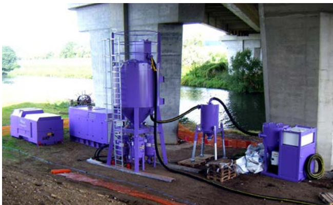
Left to right: Power and air generators, 25-ton storage hopper with a custom-engineered air-wash system installed above it, cyclone separator, MB-2000 Vacuum Unit.
