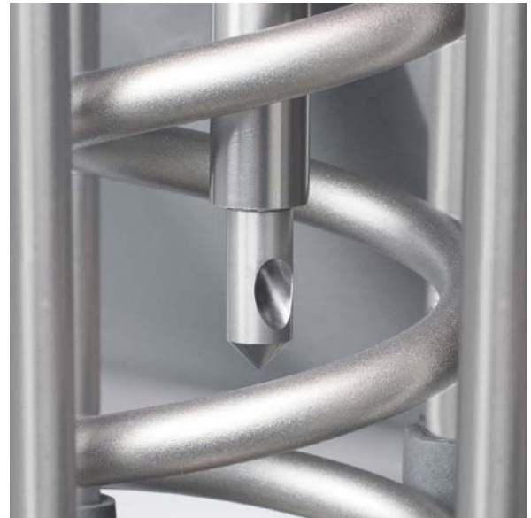
Figure 2: Lean Peening of a spring curl
