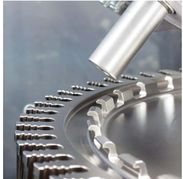
Figure 4: Peening of a turbine disk
