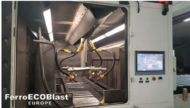
Manipulator with adjustable nozzles inside the machine
