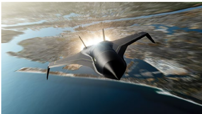
The Halcyon prototype: This Commercial Passenger Hypersonic Aircraft has a titanium alloy primary structure and 4,600 mile range
