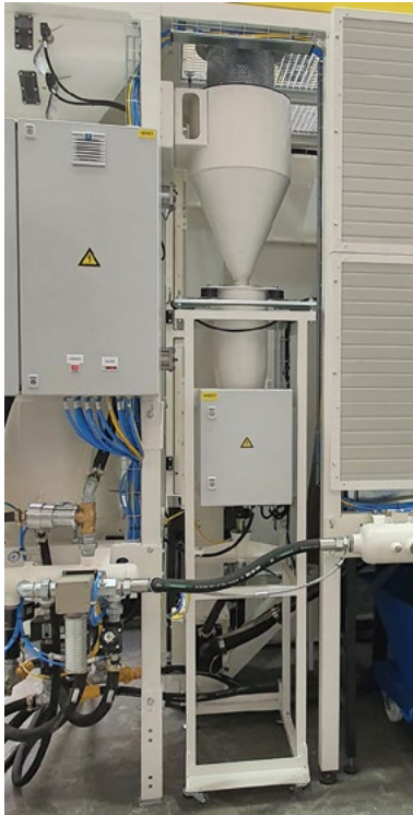
Integrated shot flow calibration system
