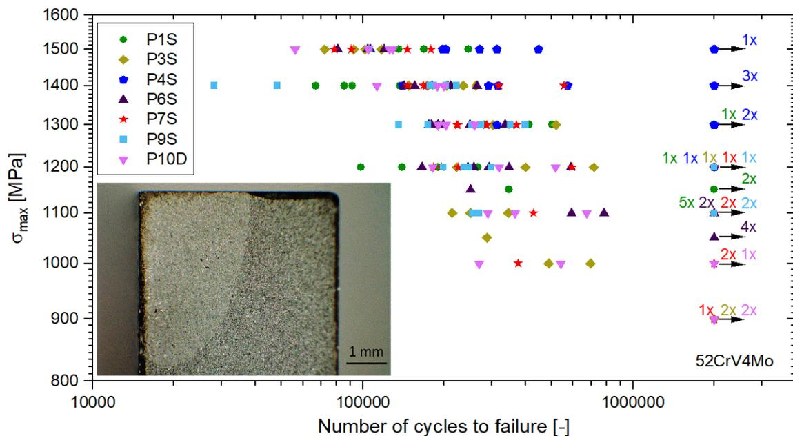
Figure 3. Overview of 4P-bending fatigue test results; edge crack (detail).
