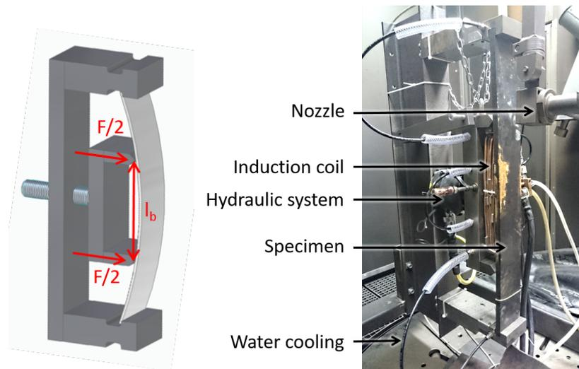
Figure 1. Schematic of 4-point bending stress peening (left) and photograph of realized warm stress peening device (right).
