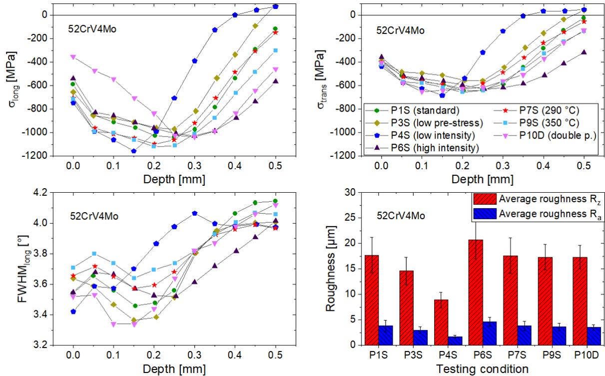
Figure 2. Top: Residual stress profiles; left side: longitudinal measurement (parallel to pre-stress); right side: transverse measurement (perpendicular to pre-stress). Bottom (left side): longitudinal FWHM profiles. Bottom (right side): Surface roughness values.
