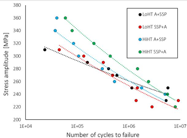
Figure 4. Results of the fatigue test in form of S-N curves. There can be seen, while in case of LoHT, no beneficial effect of introducing SSP process before aging is visible, for the HiHT series
