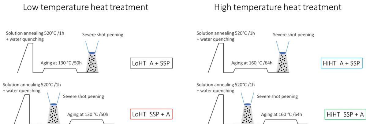
Figure 1. Schematic view of the tested sample series. Four different series were tested, differing in the aging temperature and the application of the shot peening process before/after aging treatment.
