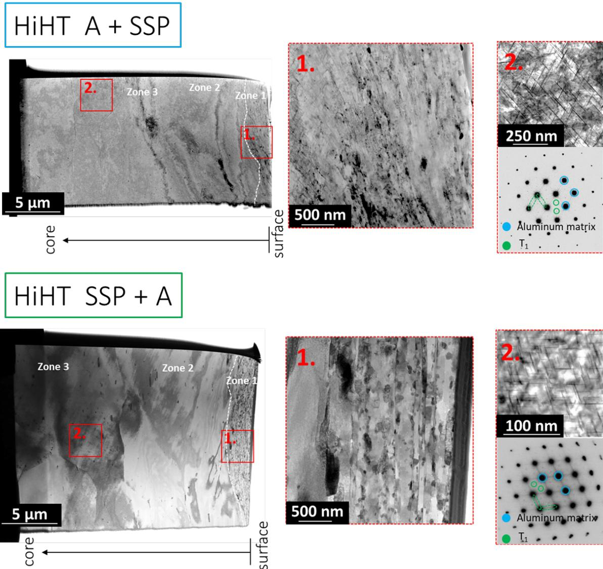
Figure 2. Microstructure of HiHT series (BF-STEM). Images showing overall view on the surface and subsurface region. Images (1) show detailed view on the nanocrystalline layer. Detailed images (2) show T1 plate-like precipitates with corresponding SAED patterns (ZA<110>).
