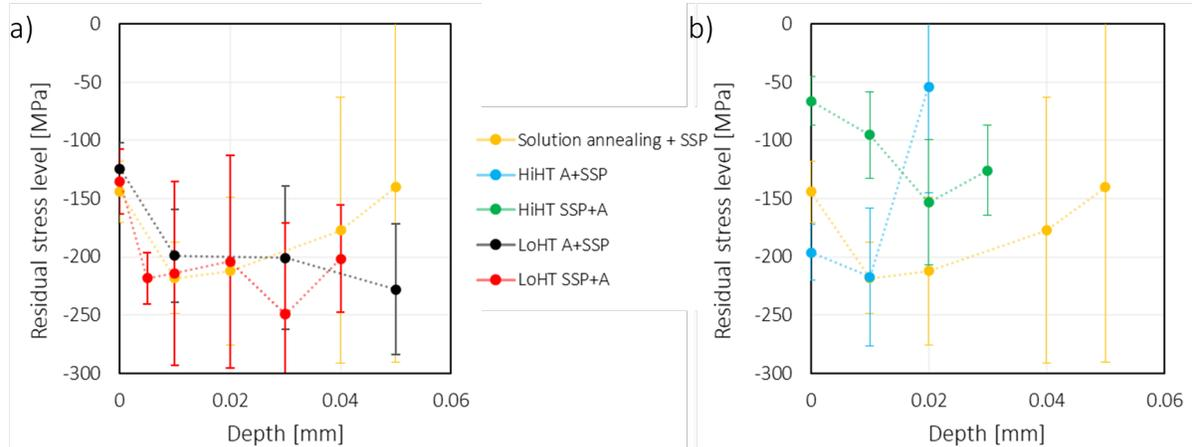
Figure 3. Residual stress depth profiles of all examined series. Compressive residual stresses in the subsurface region induced by SSP process were recorded in all series.
