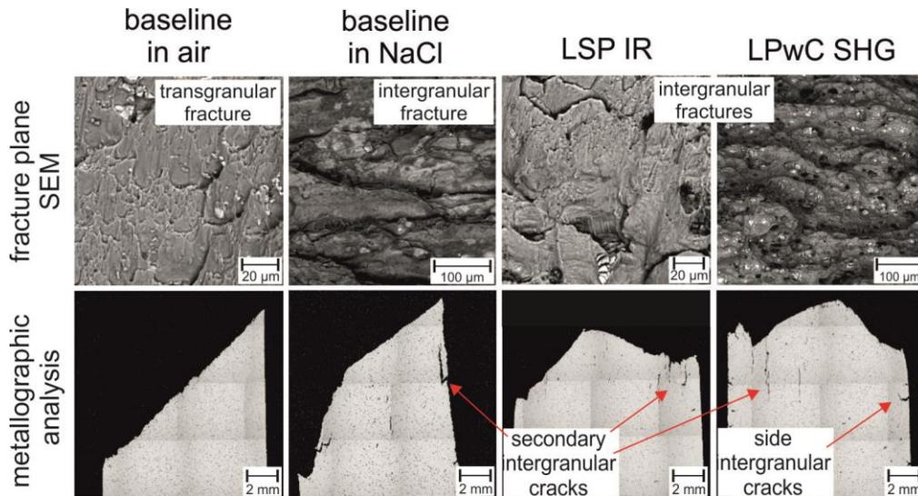
Figure 5: Fracture analysis results.
