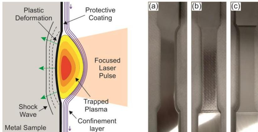
Figure 2: (left) LSP mechanism and (right) SSRT samples with (a) no laser peening, (b) LSP IR and (c) LPwC SHG.
