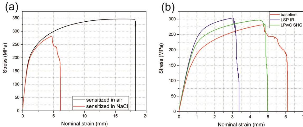
Figure 4: Stress/strain curves of (a) sensitized samples in air and 3.5% NaCl solution and (b) of sensitized samples in 3.5% NaCl solution after LSP and LPwC treatments.
