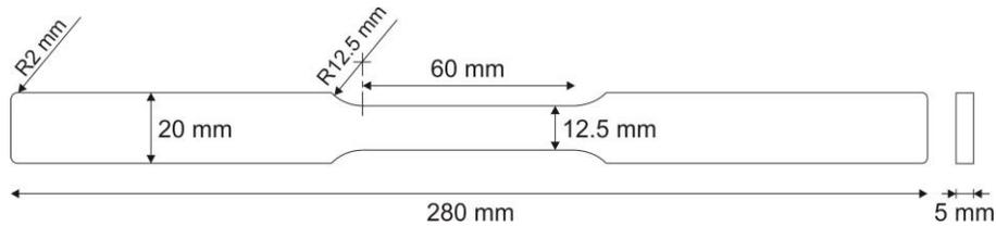
Figure 1 : SSRT sample dimensions.
