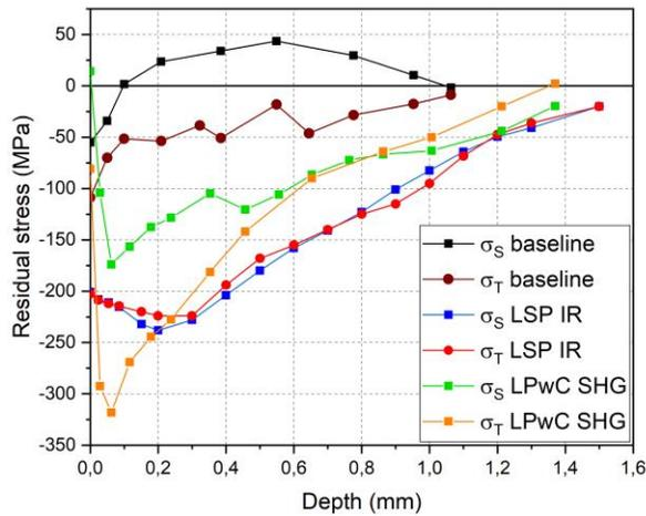
Figure 3: In-depth residual stress measurement where  $\sigma_S$  and  $\sigma_T$  denote stresses in scanning and transversal directions, respectively.
