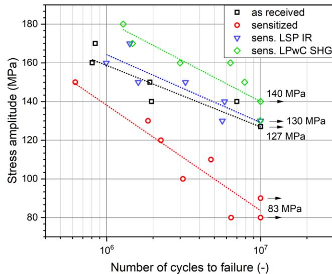
Figure 6: S-N curves of sensitized AA5083 after 3-point bend test in 3.5% NaCl solution
