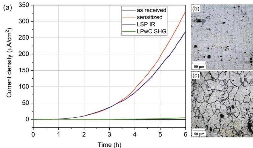
Figure 7: (a) Current density during potentiostatic polarization at  $-800 \text{ mV}$  vs  $\text{Ag}/\text{AgCl}$  electrode of non-treated and treated AA5083 in 3.5% NaCl solution. (b) as received and (c) sample surface after 6 hours of potentiostatic polarization.
