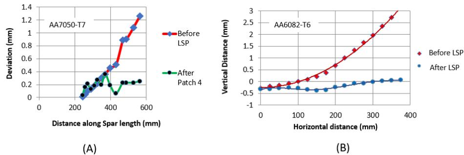
**Figure 6:** Distortion correction results before and after LSP for the AA7050-T7451 (A) and AA6082 material (B).
