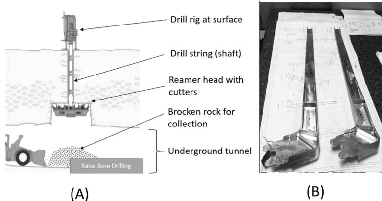
**Figure 3:** A schematic of the Raise Bore Drilling (RBD) process (A) [6], and of machined aerospace components that are scrapped due to distortion (B)
