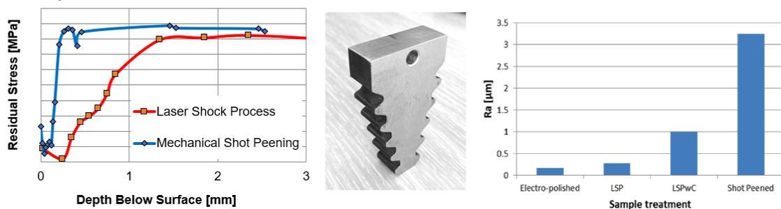
**Figure 4:** Synchrotron XRD results (left), A scale fir tree root section processed (centre), and resulting surface roughness (right) [7]
