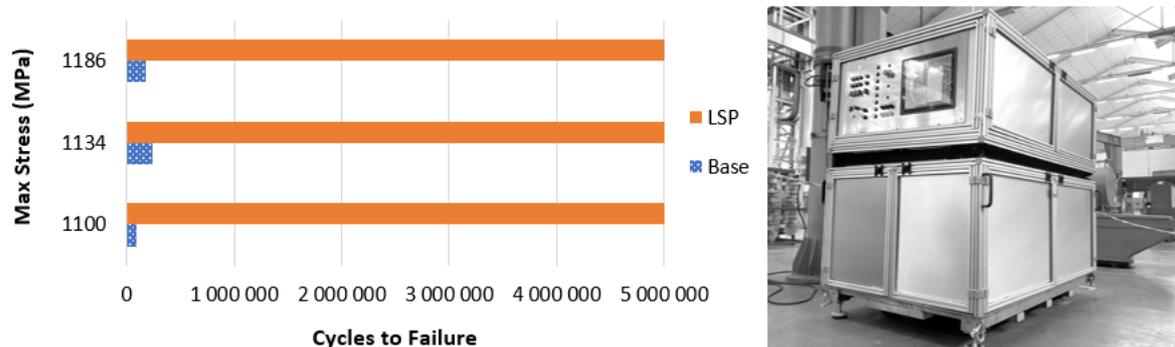
**Figure 5:** Three-point bending fatigue test results for the AISI 4330V material (left), and a photograph of the mobile laser unit under development during on-site testing (right)
