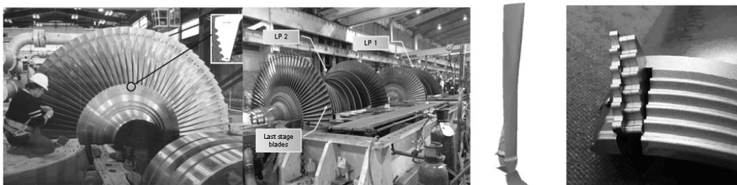
**Figure 2:** Photographs of LP steam turbine blades (left), a CAD model of a single blade (centre), and a close up of a fir attachment region after coupon removal (right) [5]
