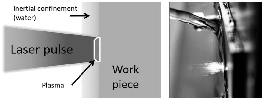
**Figure 1:** A schematic of the LSP process mechanism (left), and a photograph after the LSP process (right)
