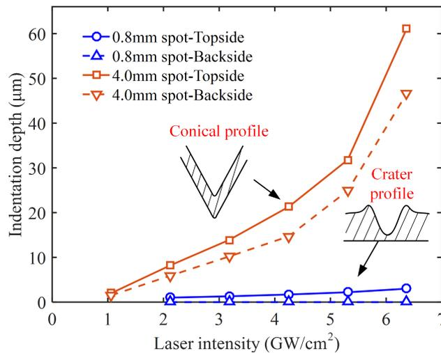
Fig. 2 Indentation depths with different laser intensities and spot sizes.
