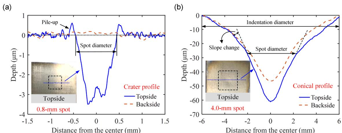
Fig. 1 Indentation profiles of specimens after a single shock with the laser power density of  $6.37 \text{ GW}/\text{cm}^2$  and spot sizes of (a) 0.8 mm and (b) 4.0 mm.
