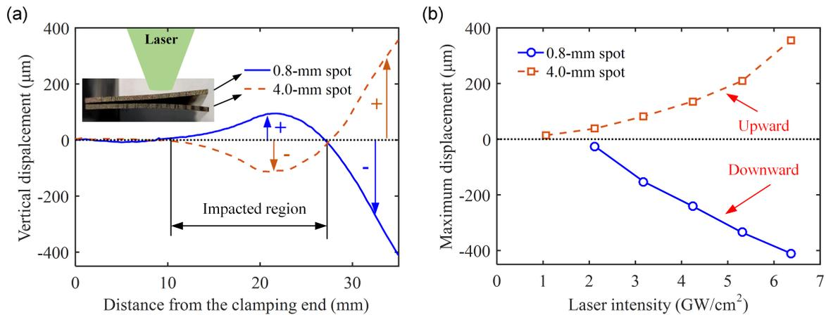
Fig. 3 Overall deformation behaviors after multiple laser shocks with different process parameters: (a) deformation profiles along the central axis under the laser power density of  $6.37 \text{ GW/cm}^2$ ; (b) maximum displacements with different power densities.
