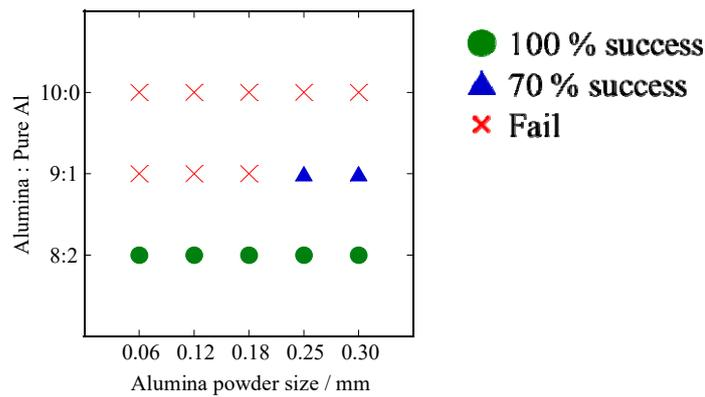
Figure 3 Bondability of laminated sheet.
