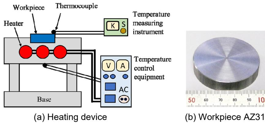
Figure 2 Equipment for bonding dissimilar material.
