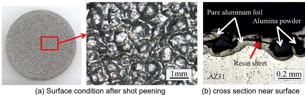
Figure 5 Surface condition and cross-section near surface.
