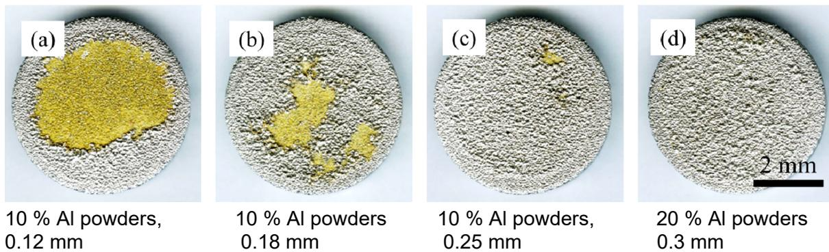
Figure 4 Appearances of shot-peened workpieces.
