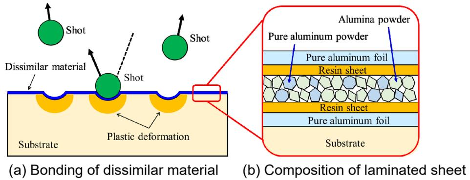
Figure 1 Bonding method of laminated sheet by shot peening.
