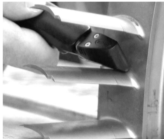
Figure 2 Pneumatic Needle Peening Application on an engine blade
