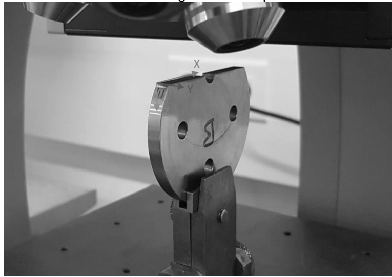
Figure 5 one side of the sample being measured to obtain the surface geometry
