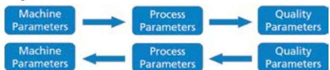
Figure 7: Reversal of simulation through AI-based determination of machine parameters from quality parameters
