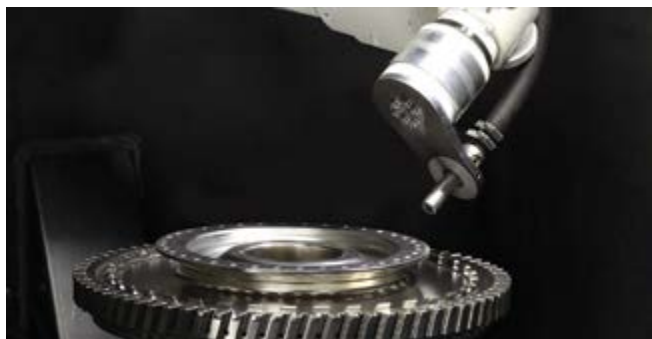
Figure 2: Spatial and temporal assignment of peening nozzle and workpiece
