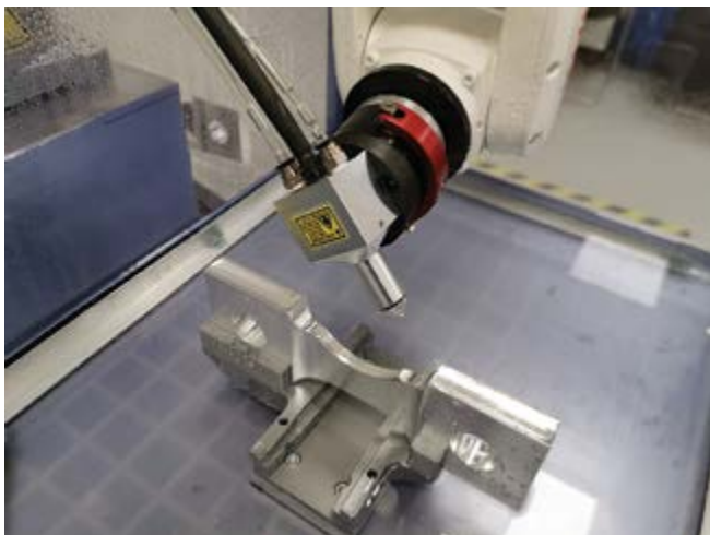
LPwC of a 3D-shaped sample by using an industrial robot.
