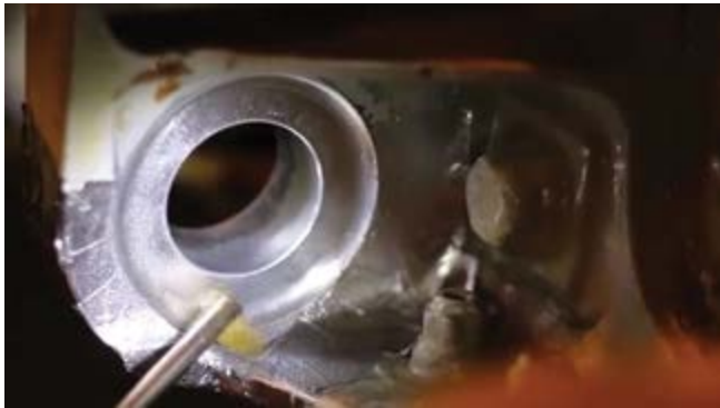
Flap peening of a pin hole
