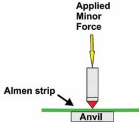
Fig.4. Applied minor force flattening pre-bowed Almen strip.
