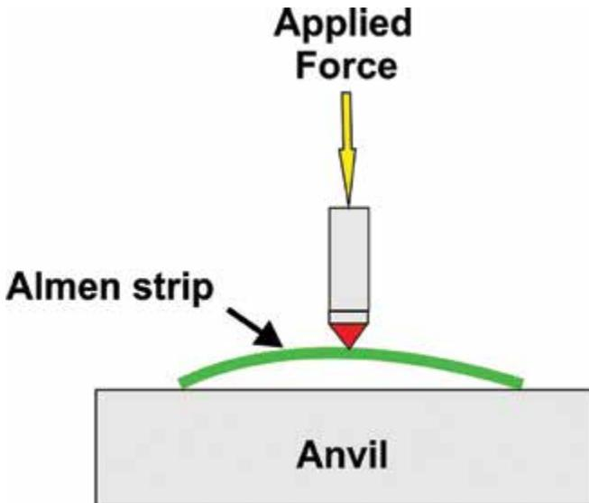
Fig.3. Rockwell indenter applied to curved-down Almen strip.
