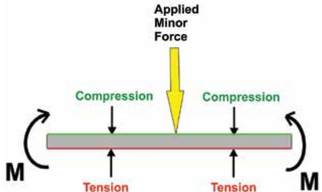
Fig.6. Stress system developed by imposing Minor Force.
