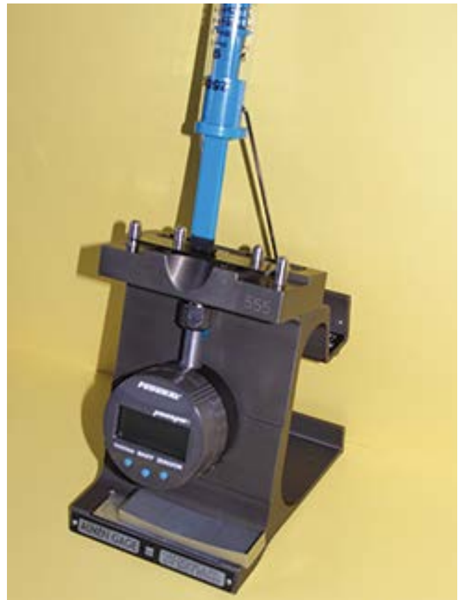
Fig.7. Device for Almen strip elastic modulus determination.
