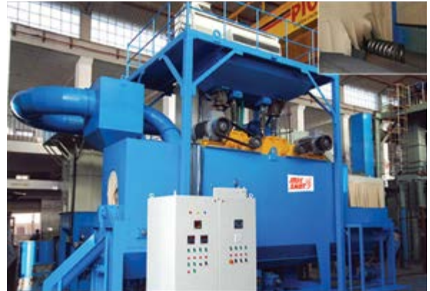
Airless wheel blast machine for the shot peening of coil springs
