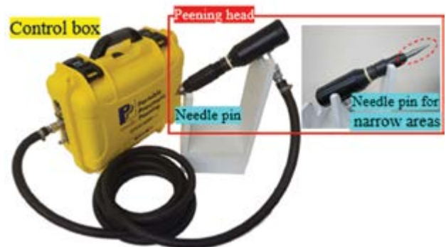
Fig.4 Portable pneumatic needle peening device
