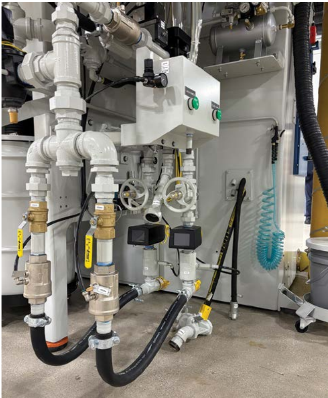
Two 600 series MagnaValves control media to two nozzles
