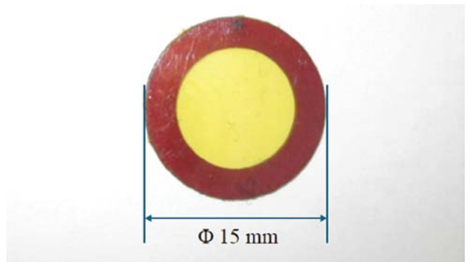
Fig. 1 Sealed ^{22}\text{Na} source supplied by JRIA
