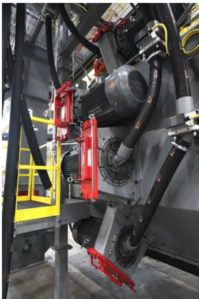
The M3A TwistLOK™ e-Wheel™ from Blast Cleaning Technologies with blade lengths upto 17.5” spins at 3600 RPM with a direct-drive motor to generate velocities upto 350 feet per second
