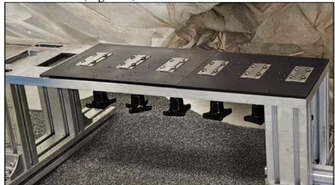
Figure 2: Almen test bench for multi-pressure setup
