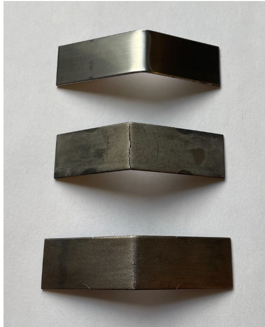
Figure 1. Post-bending photos. From top to bottom: unpeened as-received, as-peened, peened HC72h.
