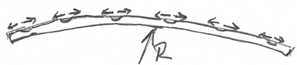
Figure 2 - Convex Bending of the Almen Strip at the Peened Surface
