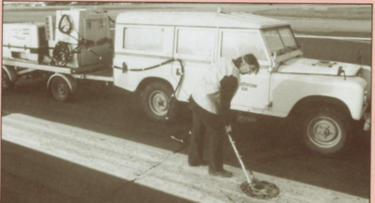
Two views of the Vacu-Blast runway light cleaner in operation.
