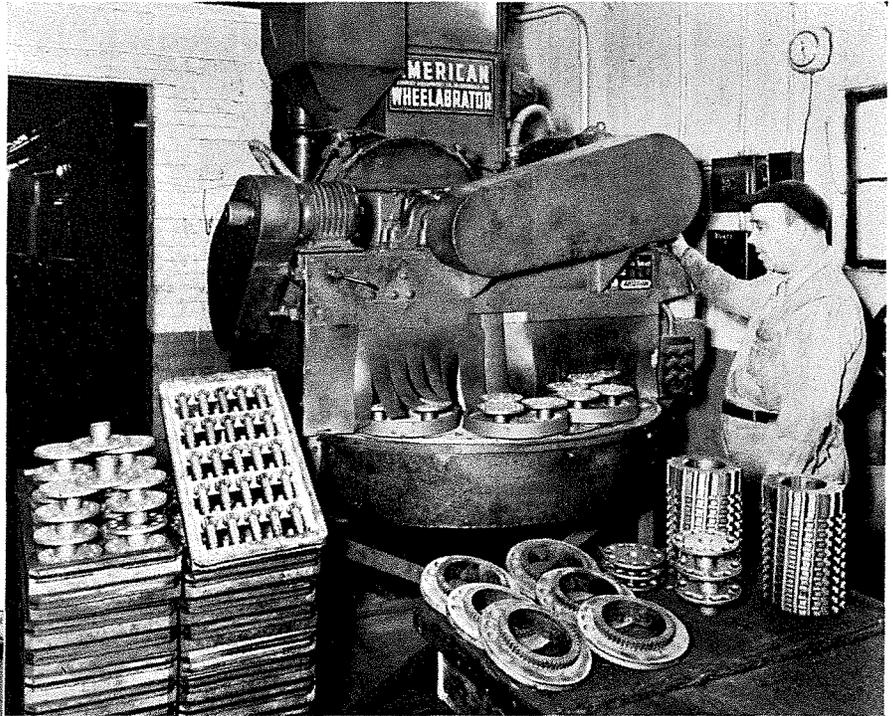
A Hartford, Connecticut, plant finds their No. 1 Wheelabrator Table invaluable for cleaning aircraft gears, heat treated parts, etc.
