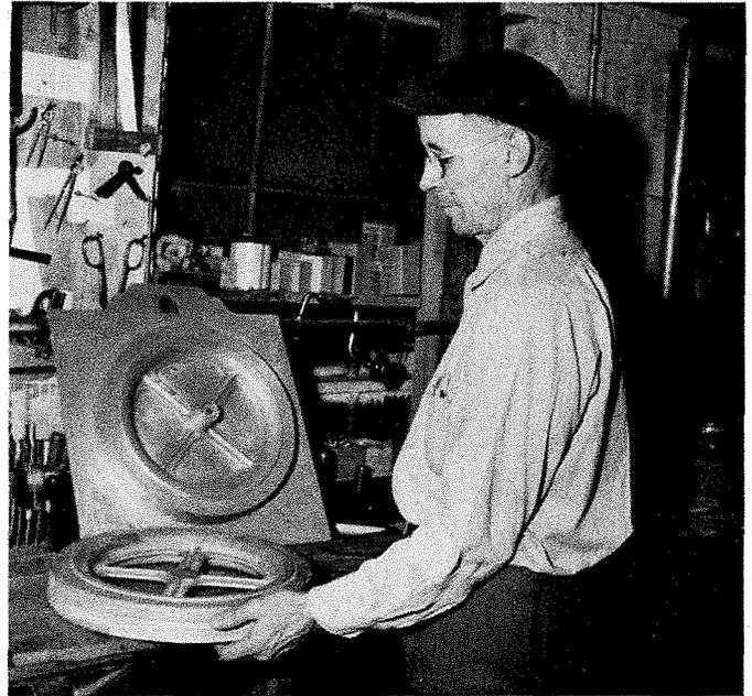
Standing in front of his workbench where various types of wood working tools are within easy reach, head pattern maker, CLAY FISHER displays a finished wood pattern and the metal pattern made from it. The metal patterns are made outside our plant from wood patterns these craftsmen produce. The plate to which this sandcutter take-up reel sheave pattern is attached fits over the molding flask, centering the form in the sand.
