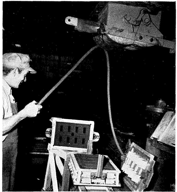
How it is used: Molder DELBERT KINNEY has finished a mold for a dust collector shaker part. The cope or top of the flask is on its side next to the drag or bottom of the flask. The metal pattern stands on its side in front of the molder. The two parts of the flask will be slipped together, then lifted off leaving the mold within the sand ready for the pouring. The same pattern and flask will be used again for the next mold.
