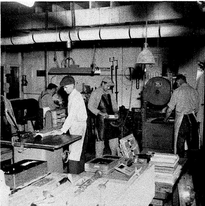
A general view of the pattern shop showing some of the wood working machinery used there. HERMAN ABLE operates the wood turning lathe. On this lathe the tool is held in the operator's hand rather than fastened to the machine. CLAY FISHER rips through a piece of wood on a band saw, ELDIEN POWELL operates a sander while LEO GORDON cuts a piece on a power saw. There are also special machines for wood shaping, planing, routing, etc.
