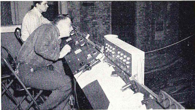
Control panels for the engineers and dispatcher. The board in the foreground is for the dispatcher. Bob and another engineer operate trains from the control panels in the balcony. Each engineer is provided with signal lights, a switch to make the train move in either direction, a rheostat for controlling the speed of the train, a time table, and an ampere indicator. The balcony is reached by climbing the regulation 19-inch railroad ladder.
