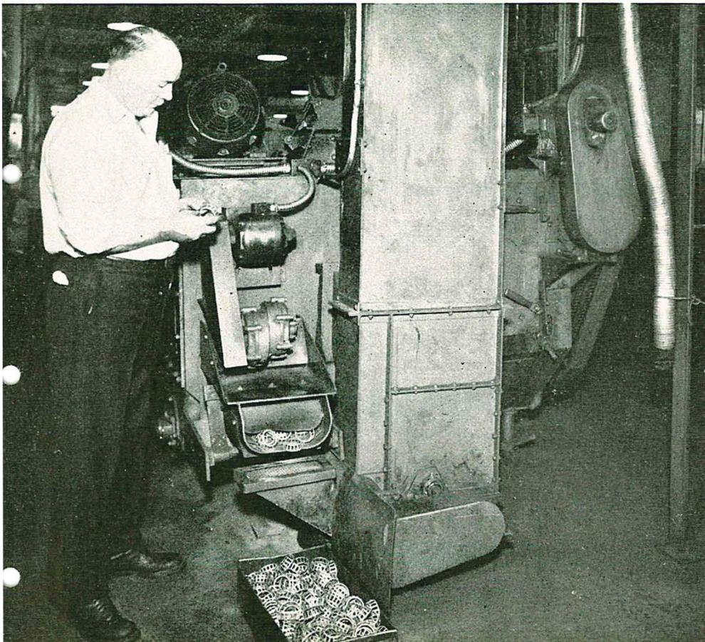
where complete exposure of the work to the full effect of the blast from one or more Wheelabrators is accomplished by tumbling the pieces in a chamber formed by an endless apron conveyor — an exclusive American development.
