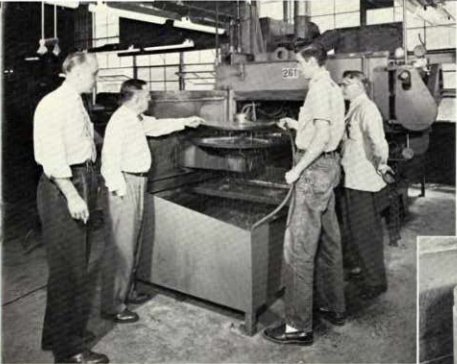
(AT LEFT) Overall view of the Special Cabinet with four Jacquard people looking on. The Plant Super intendent is pointing at the knitting machine dial which is positioned for rinsing on the Swing Table. This dial is so placed as to allow the stationary nozzle to clean the forepart of the dial.
