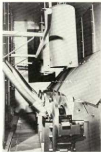
Inside the blasting apparatus of the Wheelabrator Special Cabinet. Visible are the four up-blast wheels for etching the inside of the shells.
