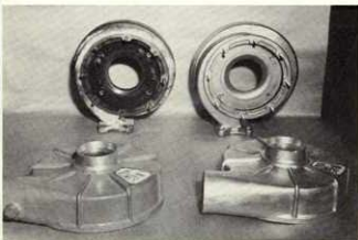
The "before" and "after" picture of a supercharger compressor casing which was Liquamated.
