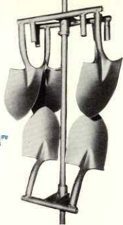
Even shovels, which are generally used in "dirty" work, can be dressed up in this manner for Wheelabrating.
