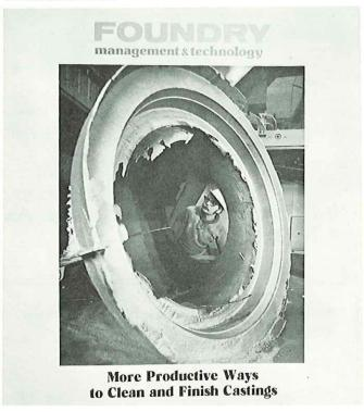
A Wheelabrator 96-inch Swing Table leads off the cover story—"More Productive Ways to Clean Castings"—in the current issue of Foundry Management and Technology. Pictured is the inspection of a large pipe elbow casting immediately after blast cleaning in our Swing Table. No-bake sand is broken up and reclaimed in the casting cleaning operation at the Backman Foundry, Provo, Utah.
