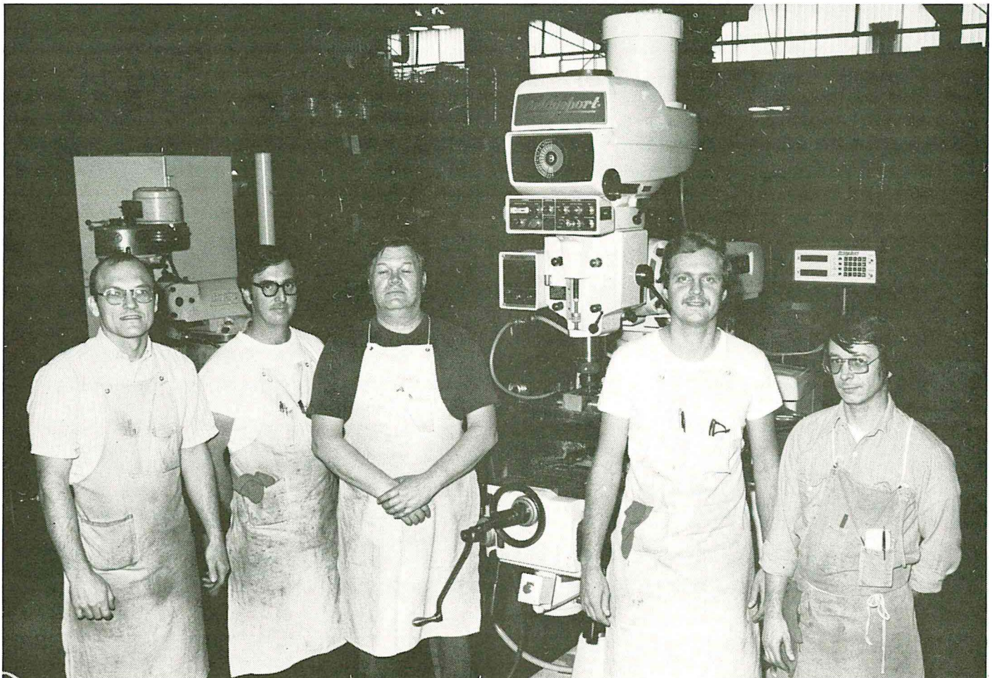
Back to us . . . one way in the purchase of modern, efficient equipment to make our jobs easier and safer. Tool Makers (l to r) Bob Stief, Don Waumans, Gene Bradley, Pat Kowalski and Jim Kite show us their new Bridgeport Milling Machine — used for the maintenance and construction of dies, jigs and fixtures. (Missing from the photo is Lenny Krueger .)
