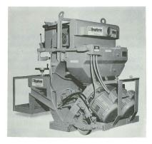
The U.S. Navy has contracted with Wheelabrator to have a 2-48 D Blastrac built and debugged, ready for shipment by **April 1, 1980**. (The 2-48 D is a two-wheel portable blast cleaning machine, with a cleaning swath of 48 inches.)
